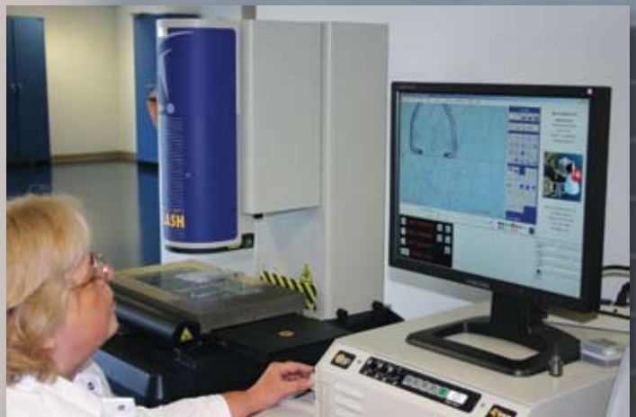
Optical measurement systems assist in accurate and fast verification.
