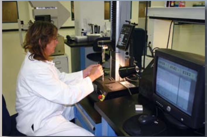
In-house capability for testing of wire and components. Here tensile testing can be performed to verify wire tensile or weld strength.
