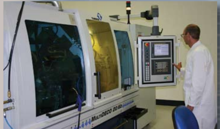
Multispindle CNC machining center for producing precision micro-components for sub-assemblies.
