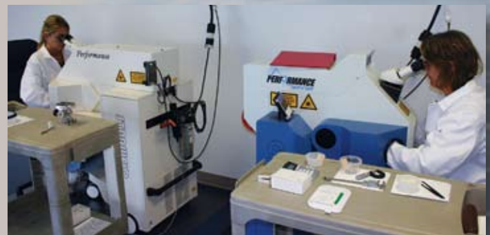
Manual laser welders assist in process development and rapid prototyping as part of our R&D activity.
