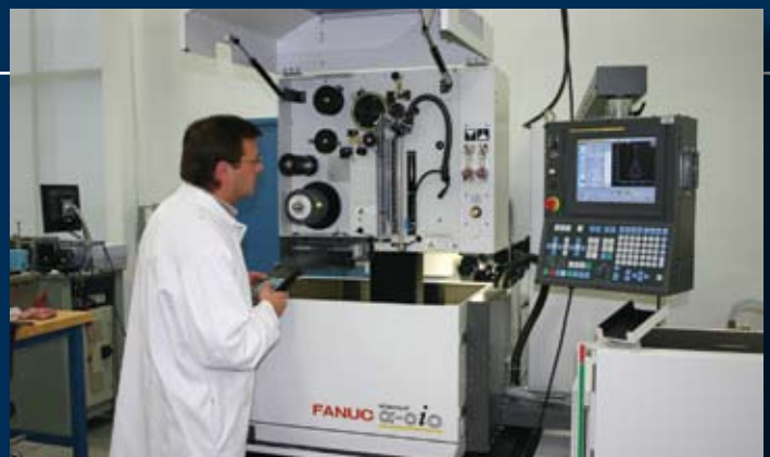
Wire EDM capability for wire cutting of precision components and for producing highly accurate tooling.
